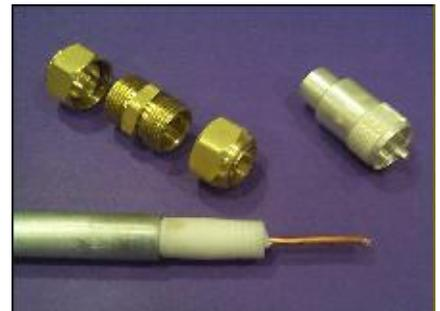
Step 1 - Shows stripped coax and required parts - a 1/2" compression union and a PL-259
