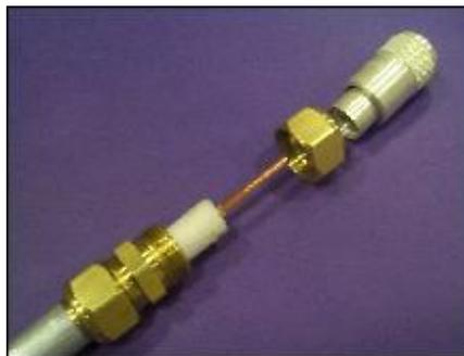
Step 4 - Push the union onto the hardline until the shield contacts the stop, then screw down the nut and ferrule you just installed.
