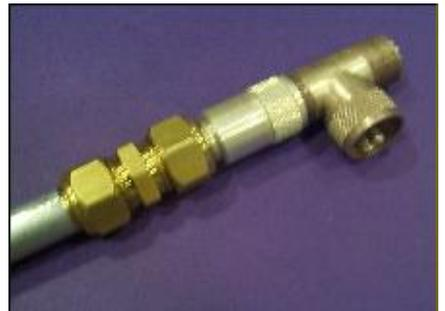
Step 5 - Add the second nut/ferrule (don't tighten yet), then use a Tee connector to screw the PL-259 onto the dielectric, leaving just enough room to loosen the PL-259 clamp nut. You'll need to trim the hardline center conductor a bit, so do a trial fit first, before tightening the second nut/ferrule. Solder the center conductor.
