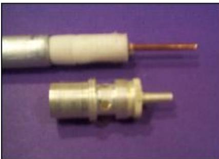
Step 2 - Use the body of the PL-259 as a length gauge when stripping the coax
