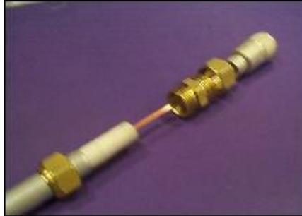
Step 3 - Push the nut and ferrule onto the coax shield Use NoAlOx and Scotchbrite to polish the shield 1 inch back from the end.
