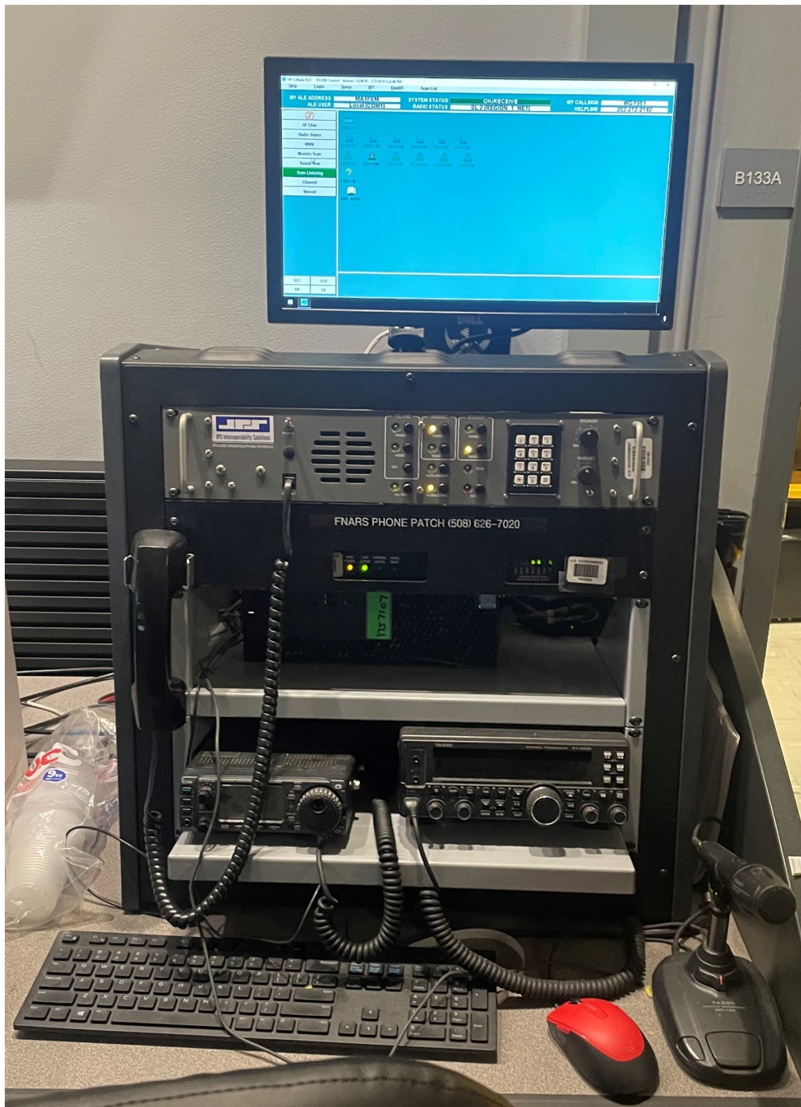
Figure 25-This is the amateur radio station in the communication room. The bottom two radios from left to right are: ICOM 706 and Yaesu FT-450D. The top radio is a user-friendly radio (i.e., don't need to be a ham) issued by the federal government.
