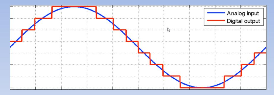
Analog-to-Digital Converter (**ADC**) measures amplitude of the input signal periodically (this is called "**sampling rate**"). 8KHz is enough for voice. The range of amplitudes (zero to max) is called "**resolution**" and is measured in bits
