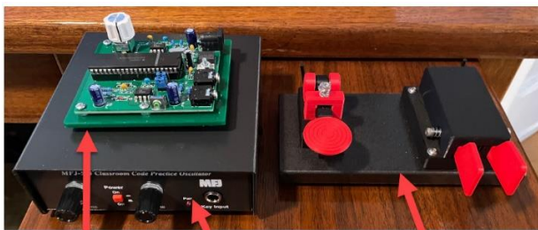
Iambic Paddle Practice Oscillator Straight Key Practice Oscillator Double Paddle Key & Straight Key with Steel Base
