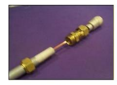
Step 3 - Push the nut and ferrule onto the coax shield Use NoAlOx and Scotchbrite to polish the shield 1 inch back from the end.
