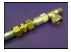
Step 5 - Add the second nut/ferrule don't tighten yet), then use a Tee connector to screw the PL-259 onto the dielectric, leaving just enough room to loosen the PL-259 clamp nut. You'll need to trim the hardline center conductor a bit, so do a trial fit first, before tightening the second nut/ferrule.
