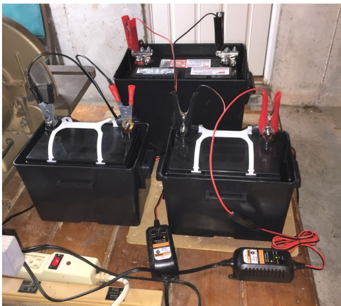
Figure 5 to left, shows our batteries being charged 24-7 with battery maintainers. A maintainer is a smart device that charges the battery constantly, but safely. It will never overcharge it, unlike some trickle chargers. A battery life is increased if it is not allowed to discharge.
